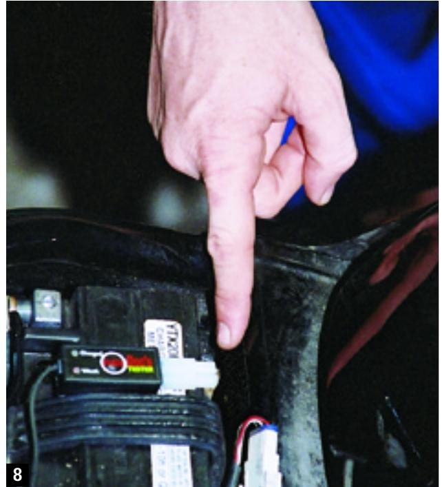
8 Now, whenever you like, you can test the condition of your battery by plugging the tester into the quick clip connector already wired to the battery. If you find that your battery does need charging, the quick clip connector plugs right into the Battery Doc.
