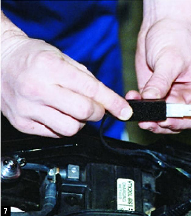
7 We connected the ring terminals to the battery, then applied one side of the hook and loop fasteners to the back of the Battery Tester and put the other side on an area that won't be seen. We chose a place right behind the battery.
